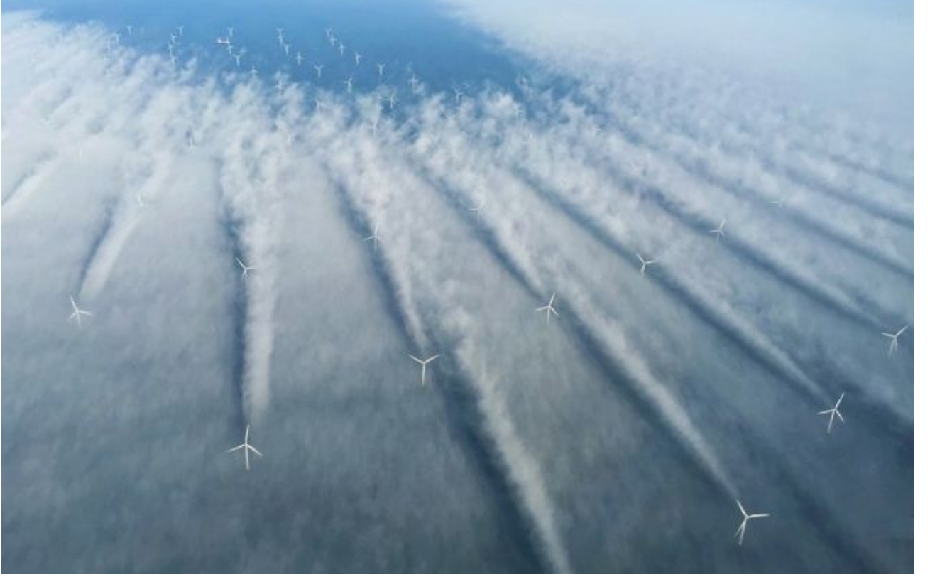
Figure 1.1: Visible wind turbine wakes in large-scale wind park (Horns Rev 2) from Dong Energy/Bel Air Aviation Denmark Helicopter Services (2017).
