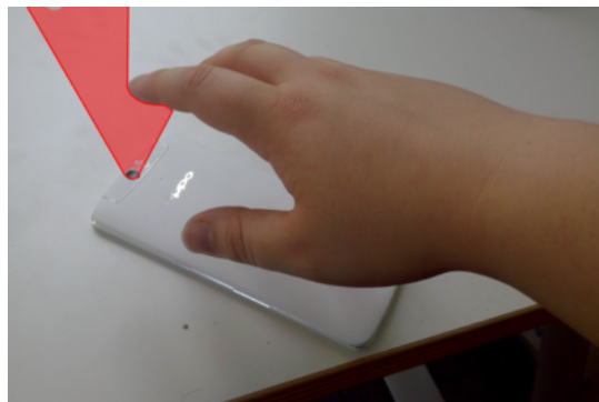
Figure 4: While a user picks up a device the right index finger moves through the rear-facing camera view-port (red). An attacker can use this moment to create an image of the user’s fingerprints.
