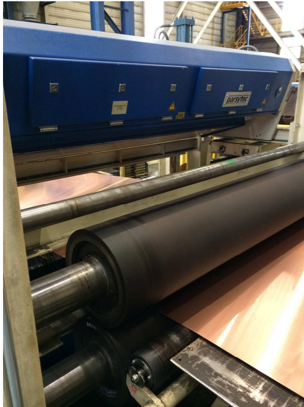
Fig. 3: ISRA Parsytec-system at a slitting and cut-to-length line for copper strip at thickness of 2 mm (source: MKM)
