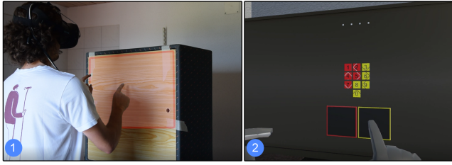
Figure 3: We mapped a physical surface in the real world (1) to the virtual screen (2) in the virtual environment. Following this approach provides users with haptic feedback when touching the screen without using an actual touchscreen.
