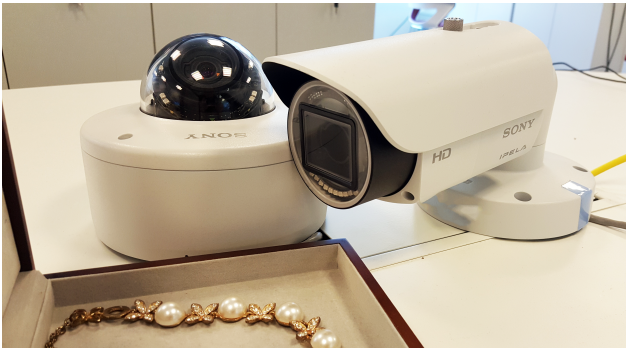
Fig. 6: Two of the cameras used in the IP camera video surveillance network. Left: SNC-EM602RC . Right: SNC-EB602R .
