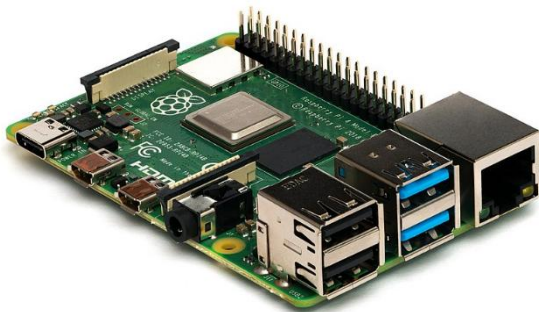
Fig. 1. Raspberry Pi 4 Model B Board
