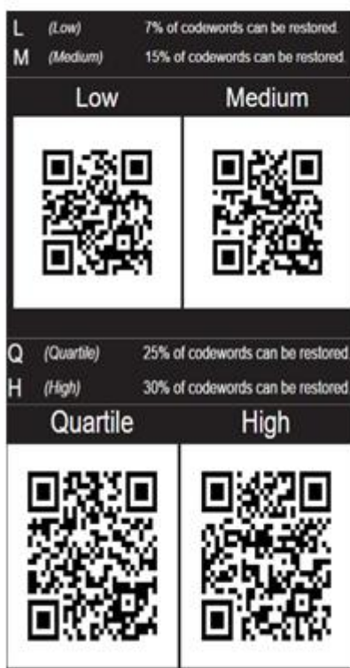
Fig 2. Efficiency of quick response code with respect to error correction
