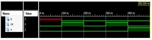
Fig. 4.4 Test bench waveforms of Shadow Latch
