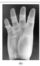
Fig. 1: 3D whole hand target for evaluating slap and contactless fingerprint readers. (a) Electronic 3D hand target complete with the four fingers, thumb and fingerless glove; the index and middle fingerprints engraved on the target are shown at full scale in red and blue boxes, respectively. (b) Fabricated hand target with translucent rubber-like material TangoPlus FLX930 [Stb].
