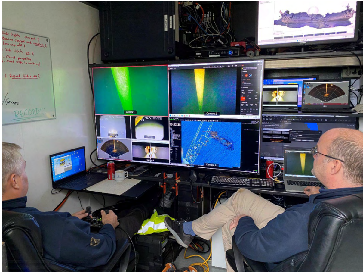
Figure 50. The experienced ROV pilot from Ocean Discovery is navigating the ROV over and around the wreck while taking photos. Photo by Anne Marie Høier Eriksen.
