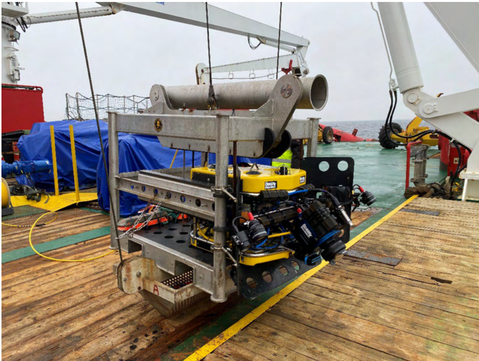
Figure 49. The ROV (equipped with cameras and lights) was prepared to be sent 150 meters down to the wreck. Photo by Anne Marie Høier Eriksen.
