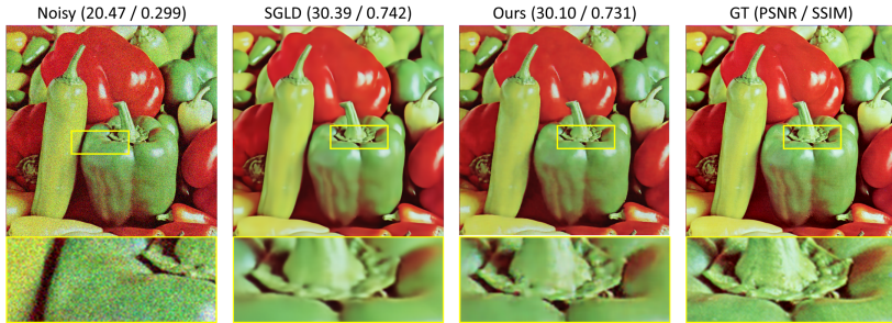
Fig. 13: Qualitative comparisons with previous DIP methods on denoising. Ours trades off the metrics for sharpness.
