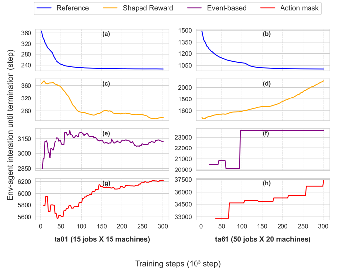
Figure 6: Ablation study conducted using "ta01" (15x15) and "ta61" (50x20) instances. (a)-(b) is the reference performance using event-based control, action-masking, and reward shaping, (c)-(d) the reward shaping is removed and replaced by a fixed reward, (e)-(f) the event-based control is omitted, (g)-(h) no action making is employed.
