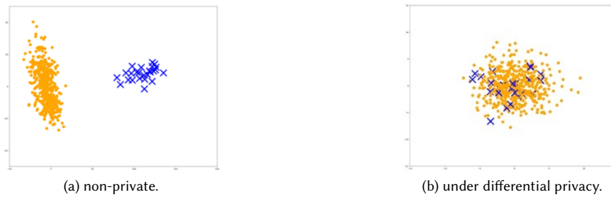
Fig. 2. PCA at the server on the local model update shared from the client on CIFAR10. The victim class is 1 (Car), and the target class is 9 (Truck). Yellow dots are benign gradient updates, and blue crosses are poisoned ones [181].
