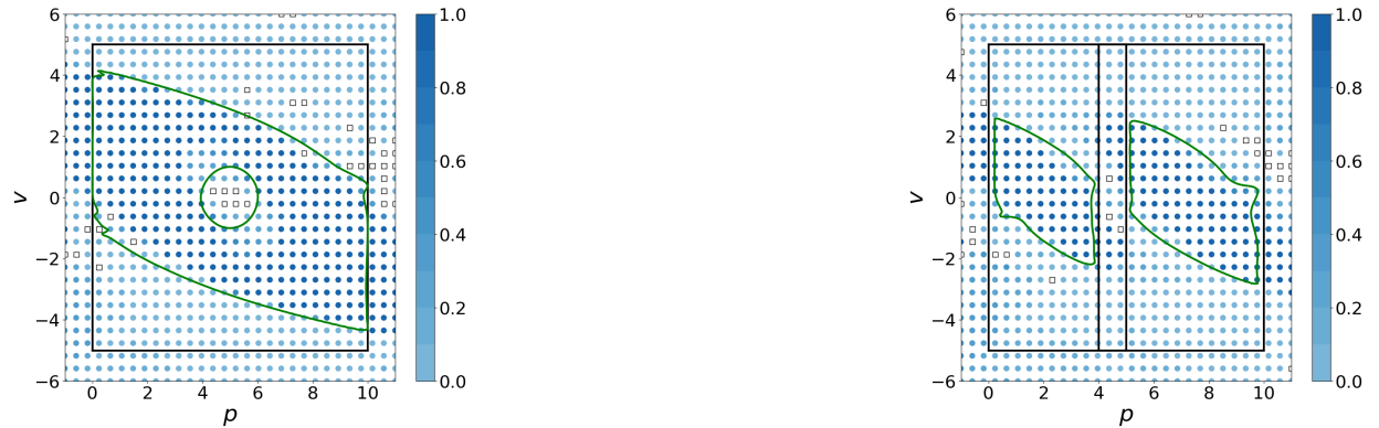
Figure 3: The 0-superlevel set of the learned NN CBF approximates the maximal control invariant set of the double integrator system in two scenarios which feature the safety constraints (p - 5)^2 + v^2 \geq 1 (Left) and 0 \leq p \leq 4 or 5 \leq p \leq 10 , respectively. The Chebyshev radius of \mathcal{K}_{\text{cbf}}(x) at each sampled state is denoted by the heatmap. States at which \mathcal{K}_{\text{cbf}}(x) is empty are marked by white squares. The black boxes denote the boundaries of the safe set in each scenario.
