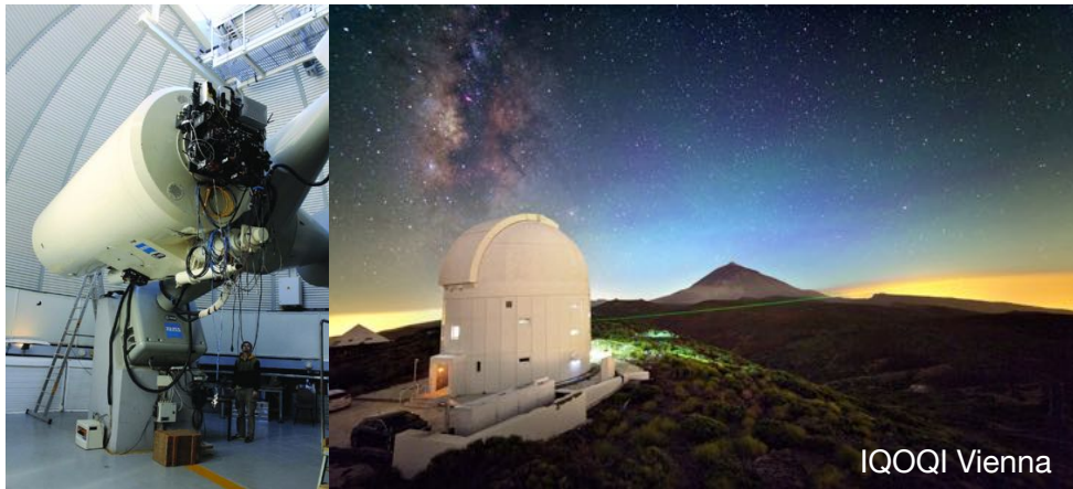
Figure 15.: Pictures of ESA's Optical Ground Station on Tenerife, configured as a quantum communication transceiver. (Images by IQOQI Wien, retrieved from https://www.esa.int/ESAMultimedia/Images )
