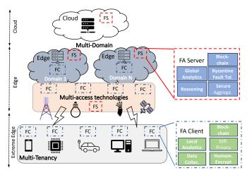
Fig. 2: Federated Analytics for 6G Architecture
