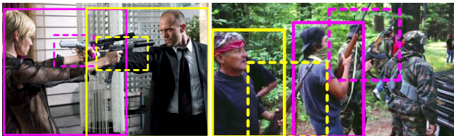
Fig. 5: Failure cases: Objects too far from the carrier in the presence of another human may result in failure of association. Likewise for overlapping firearms and occluded humans.
