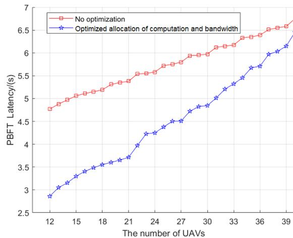
**Figure 9.** The relationship between block latency and the number of UAVs.
