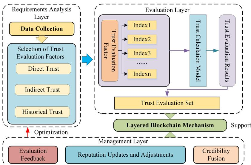
Figure 2. Trust metric model of unmanned aerial vehicle cluster nodes based on hierarchical blockchain.
