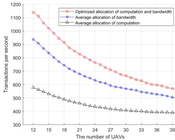
Figure 10. The relationship between the number of UAVs and the performance of our system.
