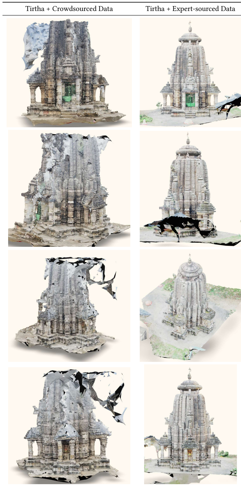
Figure 6: Gopinatha Temple: Comparing Tirtha reconstructions on different datasets. No expert-sourced mesh was available for this temple.
