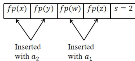
Figure 3. Marking of elements on a bucket in the position-aware Cuckoo filter.
