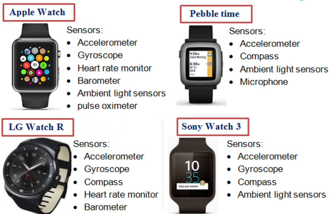
Figure 2: The existing sensors in smartwatches
