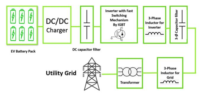
Figure 3. Fast bidirectional charger schematic for EV charging stations.
