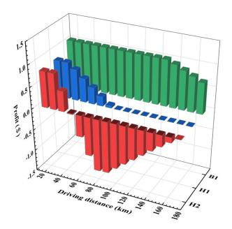
Figure 9. V2G energy scheduling mode with driving distance [84].
