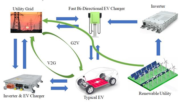
Figure 2. G2V and V2G power flows block diagram.
