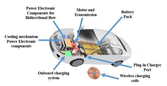
Figure 1. Conceptual EV structure and components.
