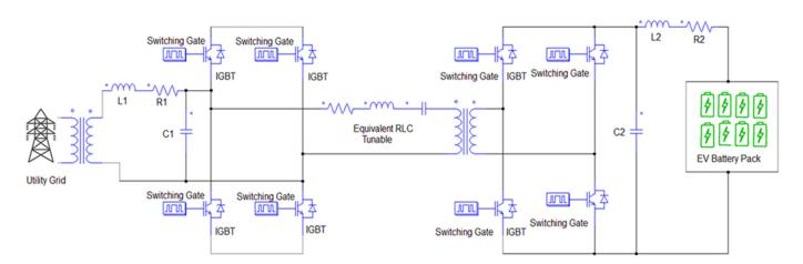
Figure 7. Bidirectional dual active full-bridge converter adoption.
