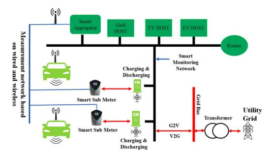
Figure 6. Smart meter architecture for bidirectional energy measurement on EV applications.
