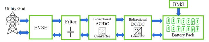
Figure 5. Uni-directional and bi-directional power flow for typical EVs.
