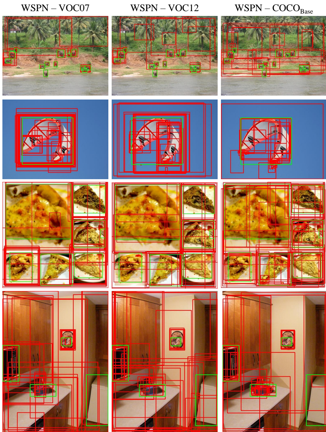
Figure 8. Qualitative analysis of WSPN network trained on VOC 2007 (20 categories), VOC 2012 (20 categories) and COCO Base 2017 (48 categories) using image-labels in a weakly-supervised manner and tested on COCO 2017 (80 categories). Here, the WSPN trained on VOC 2007 and VOC 2012 has not seen categories such as "Pizza", "Kite", "Clock" etc during training. Still, we can observe the VOC trained WSPN network can localize these unseen categories similar when tested on COCO 2017. This is due to weakly-supervised training, where the WSPN network learns to localize the object irrespective of categories it is trained on. As a result, the WSPN network trained on VOC is able to localize COCO object categories which are not seen during training. This show the generalization capability of the WSPN model and can be used to localize any objects for different dataset. Green: Ground truth bounding box, Red: Top 50 WSPN proposals.
