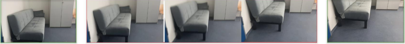
Figure 10. A self-captured sequence of frames with a smartphone. We show that two non-blurry frames on the left and right are apart by > 20 frames, where motion blur is measured using the variance-of-Laplacian thresholding. We show three sample frames in between that are affected by the motion blur. Hence, low FPS registration would have real-world use in scenarios where frames not affected by motion blur must be considered for registration.
