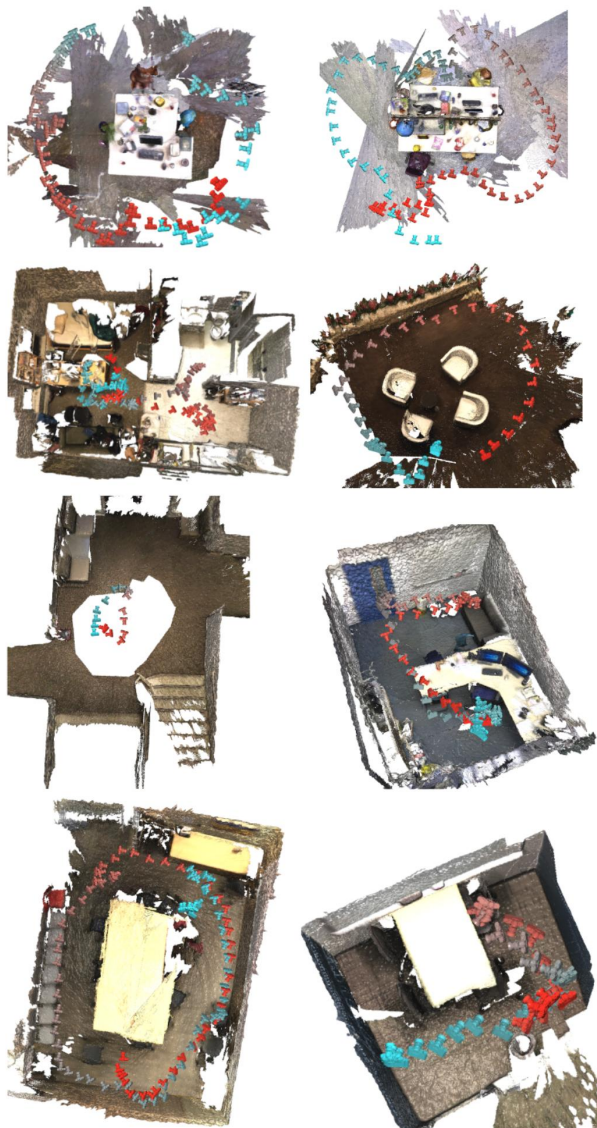
Figure 9. Example scene reconstructions from TUM RGB-D [41] and ScanNet [9] with optimized camera trajectories. Interpolation of camera color from blue to red represents the temporal order of cameras. Geometric reconstructions are obtained using scalable TSDF volume integration [8, 50].
