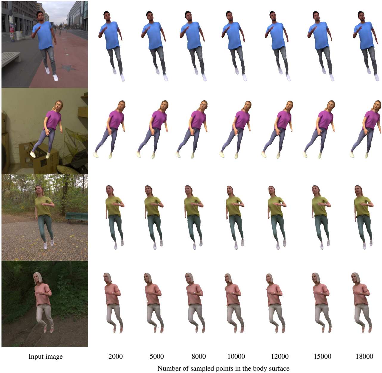
Figure 19. Qualitative ablation of number of points sampled in the body surface , storing 3D Features. Our final model has 18000 points which provides the best tradeoff between GPU memory and sharpness. Lower number of points do not affect significantly quantitative results but are less capable of representing high-frequency details.
