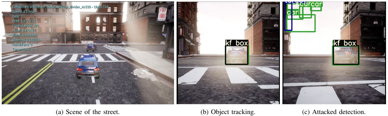
Fig. 14: The autonomous car follows the front car as shown in (a) using a Kalman filtered bounding box denoted as kf box in (b). The attacker adds image perturbations to place new bounding boxes as shown in (c).
