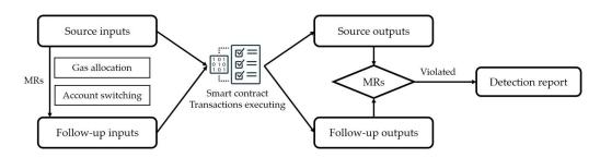
Figure 1. Overview of applying metamorphic testing to detect smart contract vulnerabilities
