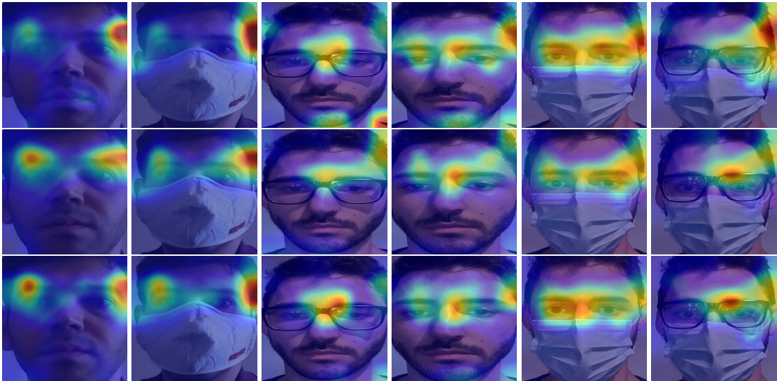
Figure 10.4: Explanations obtained for each trained model with the Smooth Grad-CAM++ explainability tool (top row images were computed from the cross-entropy model - CE; middle row images were computed from the triplet loss model - CE + TL; bottom row images were computed from the adapted triplet loss model - CE + Adapted TL).
