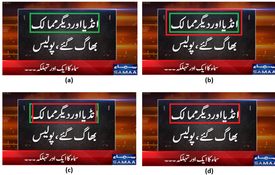
Figure 11: Computation of precision and recall (a):Ground Truth Bounding Box (b): Detected region is larger than ground truth (c):Detected region is smaller than ground truth (d):Detected region overlaps perfectly with the ground truth
