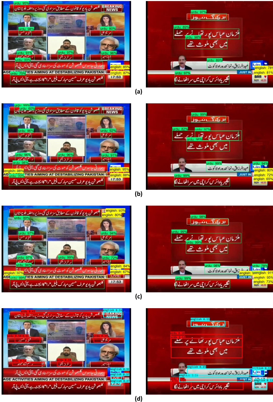
Figure 14: Detection output of hybrid text detection and script identification for different detectors (a): SSD (b): R-FCN (c): Faster RCNN (d): Yolo
