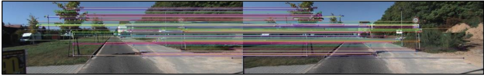
Fig. 2. The output of brute force feature-matching algorithm using SIFT features. Each match is highlighted in a random colour.
