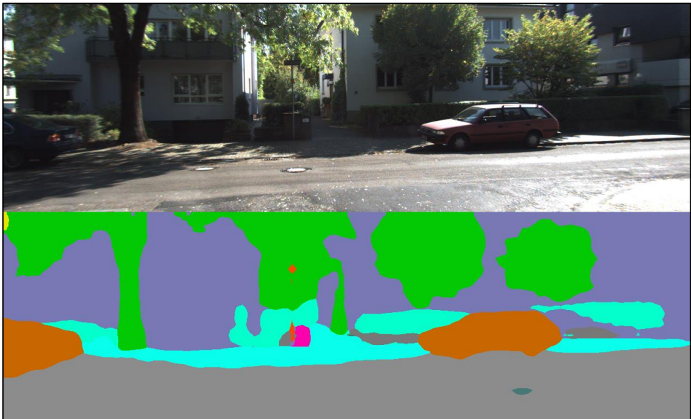
Fig. 3. Example of an image before and after semantic segmentation with a ResNet50 model. The base image is shown above. The output is shown below, with each pixel shaded in a different colour based on a class label with the highest probability.
