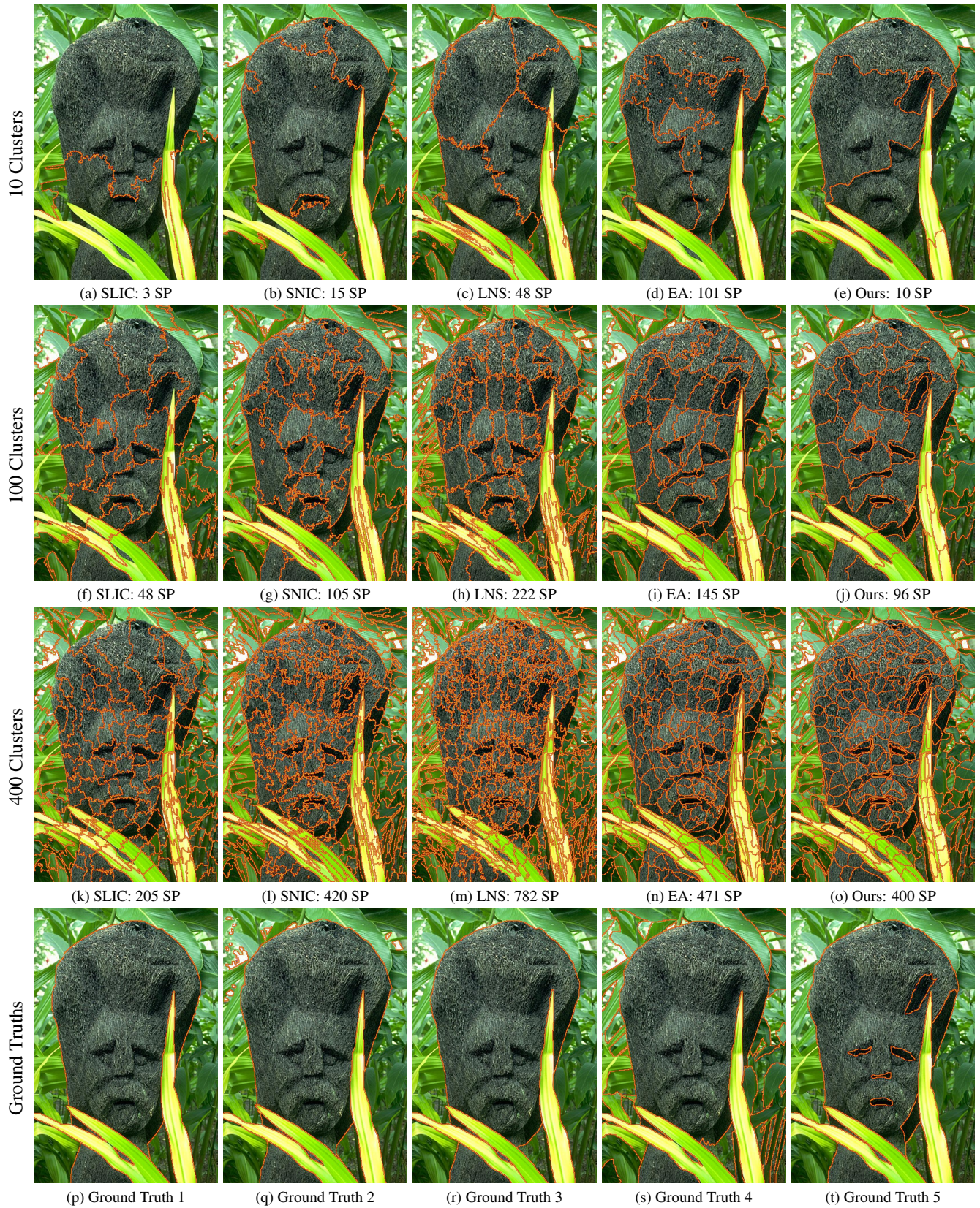
Figure 5. Qualitative Comparison of Superpixel Algorithms on a sample image from BSDS 500. The algorithms were given the cluster parameters 10, 100 and 400 (row-wise) and the produced oversegmentations are shown with the actual number of generated superpixels (SP).
