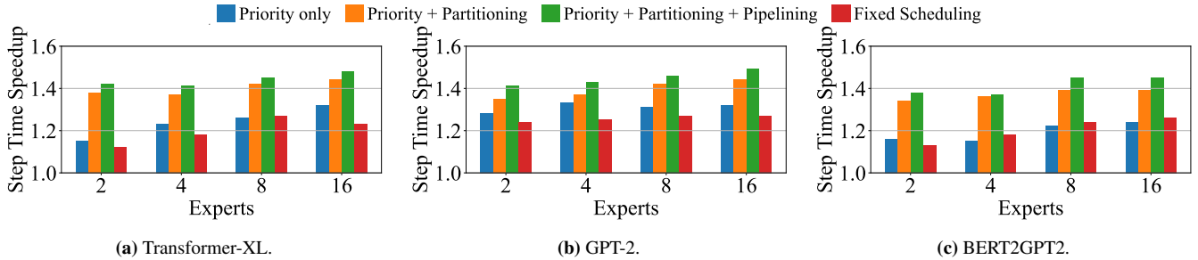
Figure 14: Speedup of training step time over Baseline with different design choices of the communication scheduler.
