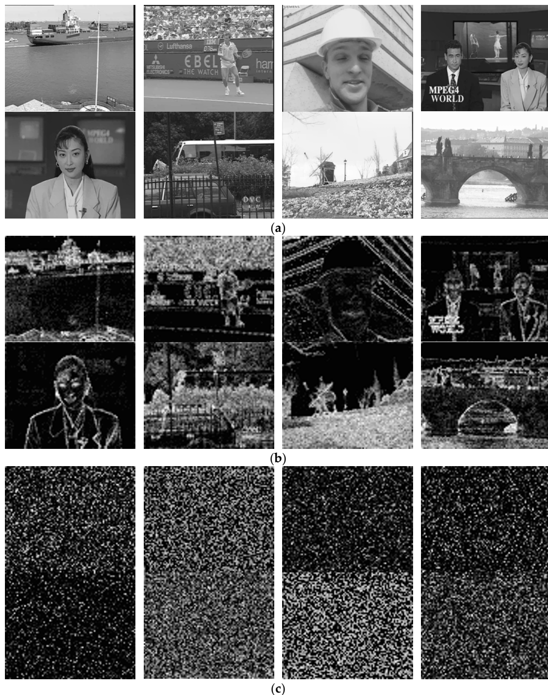
Figure 10. Effect of resisting sketch attack. (a) Original frame, (b) I-Q-M encryption, (c) proposed encryption.
