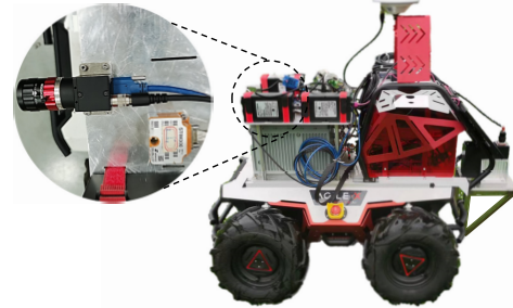
Fig. 5. We evaluated our proposed learning based VIO model with our own ground-vehicle platform equipped with RGB camera, IMU, and GNSS/IMU system.
