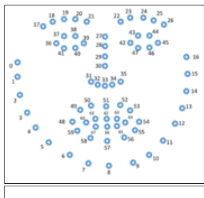
Fig. 37.2: (a) 68 facial landmark points on a human face. (b) The unit vector defined along the nose. The first three primary vectors are also shown to the centers of the eyes and mouth as well as secondary vectors from the left eye center.
