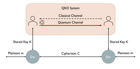
Figure 3: Generalization of the QKD system architecture.
