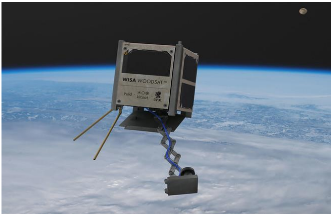
Figure 14. WISA WoodSat, a wooden satellite. Credit: Arctic Astronautics.
