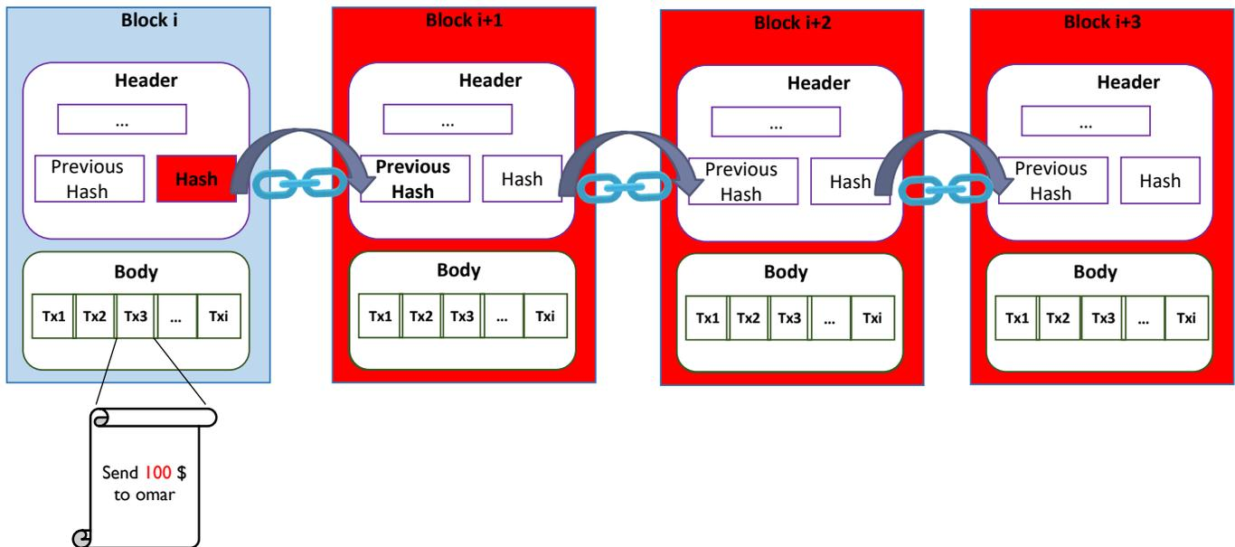
Fig. 3: Blocks are cryptographically linked, which makes them immutable
