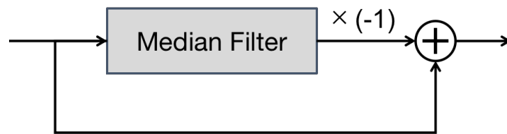
(a) A median filtering residual block (MFR)
