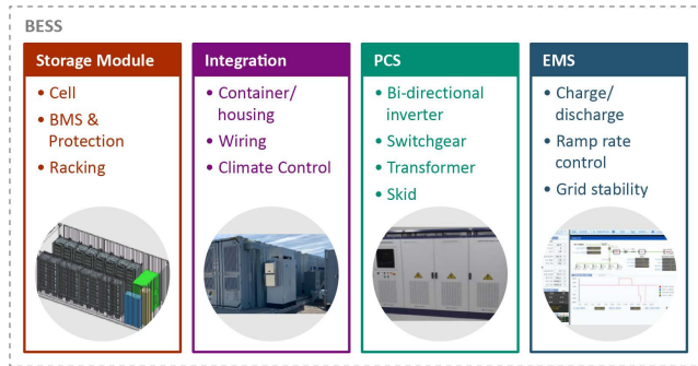
FIGURE 10. Basic elements of a utility-scale BESS [137], [138].
