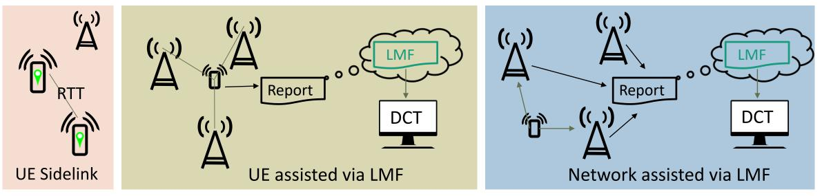
UE: User Equipment | RTT: Round-Trip-Time | LMF: Location Management Function | DCT: Digital Contact Tracing
