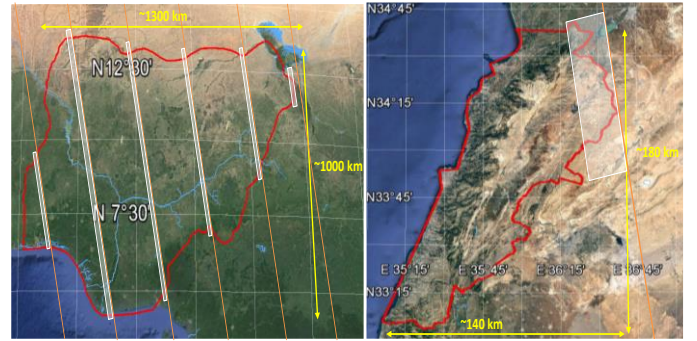
Fig. 28. Coverage scenario of Nigeria (left) and Lebanon (right) including necessary orbits and first data-take beams. (Maps from Google Earth)
