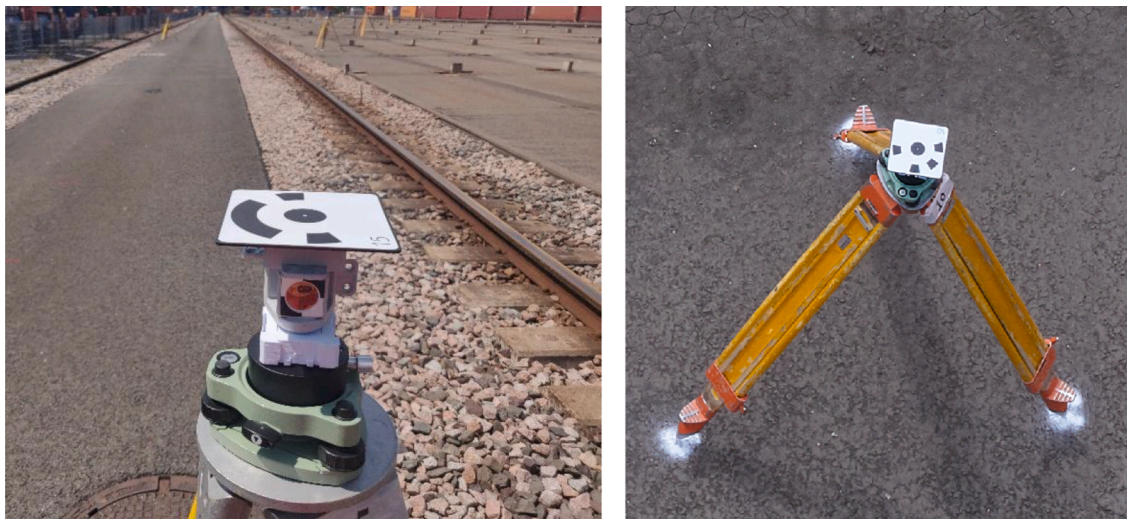
Fig. 8. High-precision reflector for tachymetric network survey integrated with a coded target for photogrammetric processing: left terrestrial view, right: image from UAV-based acquisition @ GSD = 0,9mm (Ghassoun et al., 2021).
