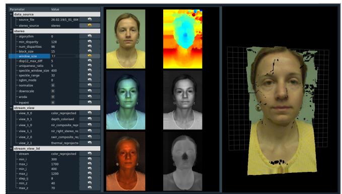
Fig. 6. Interface developed for visualizing the alignment procedure. The best calibration and parameter tuning can be selected based on this tool. On the right side of the interface, any channel (here RGB) can be projected in 3D and then after rectification reprojected to get same alignment between all channels.
