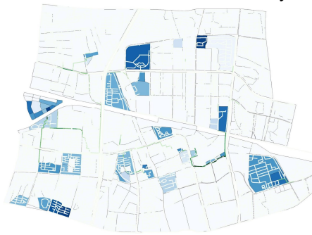
Fig. 3. Baseline scenario simulation of walking behaviour: the blue plots show the number of users per hour in a work-day; the green lines show the traffic volume over the walking network.
