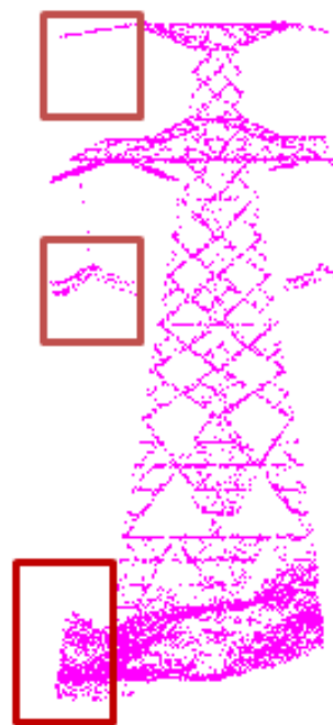
Figure 3. Noise points of transmission tower.
