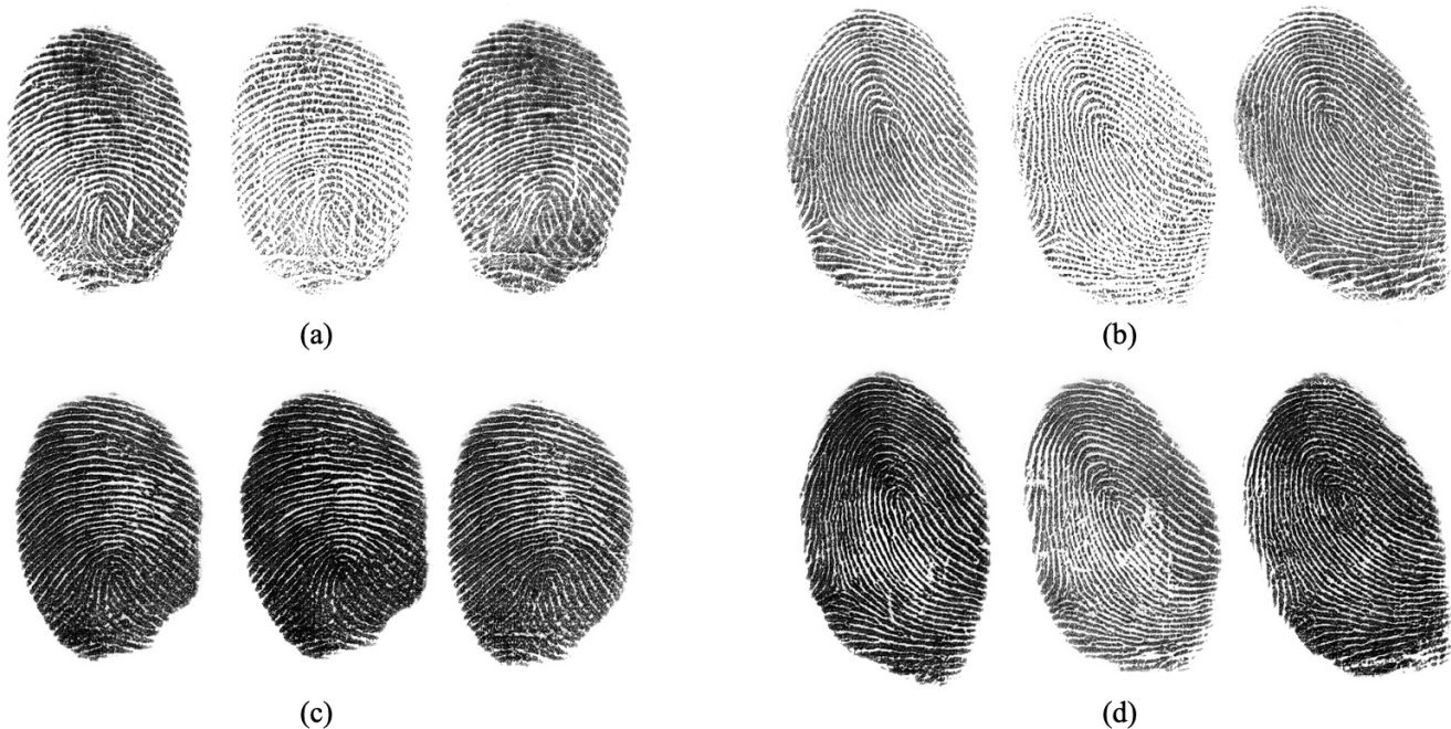
Fig. 4: Example images of multiple impressions of the same finger generated by SpoofGAN. (a) and (b) show three impressions each of two fingers rendered in a live style, whereas (c) and (d) show three impressions each of the same two fingers in a spoof style (ecoflex and body double, respectively).
