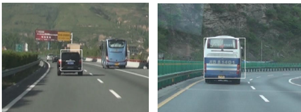
FIGURE 5. Identification results of the preceding target vehicle
