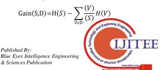
Here S is the actual set and D is the split V is the subset of S. The best split can be identified using information gain.
