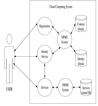
Figure 1: General Process Flow for authentication System
