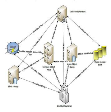
Figure 3 : Overall Interactions within Key Modules
